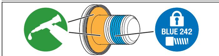
To properly assemble the Enduro, grease the surfaces of unthreaded bolt shafts, and spacers that interface with bearings (highlighted ORANGE). Follow the specific order as listed below:
