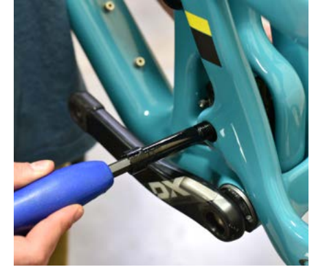
06. Lower the swingarm and re-install your Main Pivot Collet Bolt prepped with Blue 243 Loctite.
